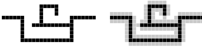
Figure 3: A one-way unit, allowing signals to travel from left-to-right but not from right-to-left. On the left the unit is shown in its unsheathed form, while the version on the right is sheathed. One gate is turned on to block the signals, another is used to prevent later signals from turning the gates off. Black cells have state 1, while grey cells have state 2 and white cells are the background, state 0.
