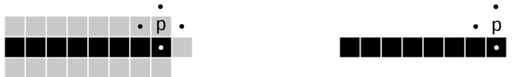
Figure 4: One reason for the sheathing is that it disambiguates certain situations. At the ends of wires, for example, it helps to distinguish a 'shoulder' cell 'p' from the cell just beyond the end of the wire, or one lying anywhere alongside a wire.
